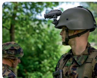
Helmet mount with auto shut-off when flipped up
